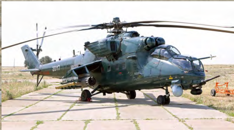
For QRA duties this Mi-35M is fully armed and ready to go in eight minutes from scramble alert; this Mi-35M is carrying the 'Baryer' system which fires RV-2 anti-tank missiles up to a range of 7500 metres.
