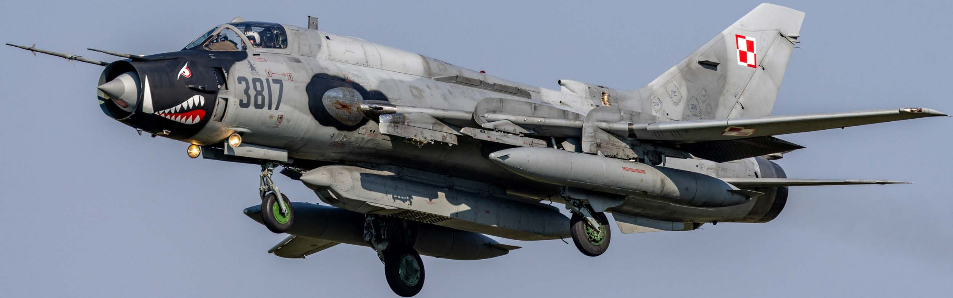
Main: After a reconnaissance mission, No. 3817 comes in for landing. Two distinctive features are immediately noticeable: the "Wild Boar" livery and the large KKR-1 reconnaissance pod Left: The aircraft on its final descent, gently gliding over Runway 25 in preparation for landing Right: The aircraft makes firm contact with the runway, leaving behind a visible trail of rubber, the signature of a well-executed landing under high load
