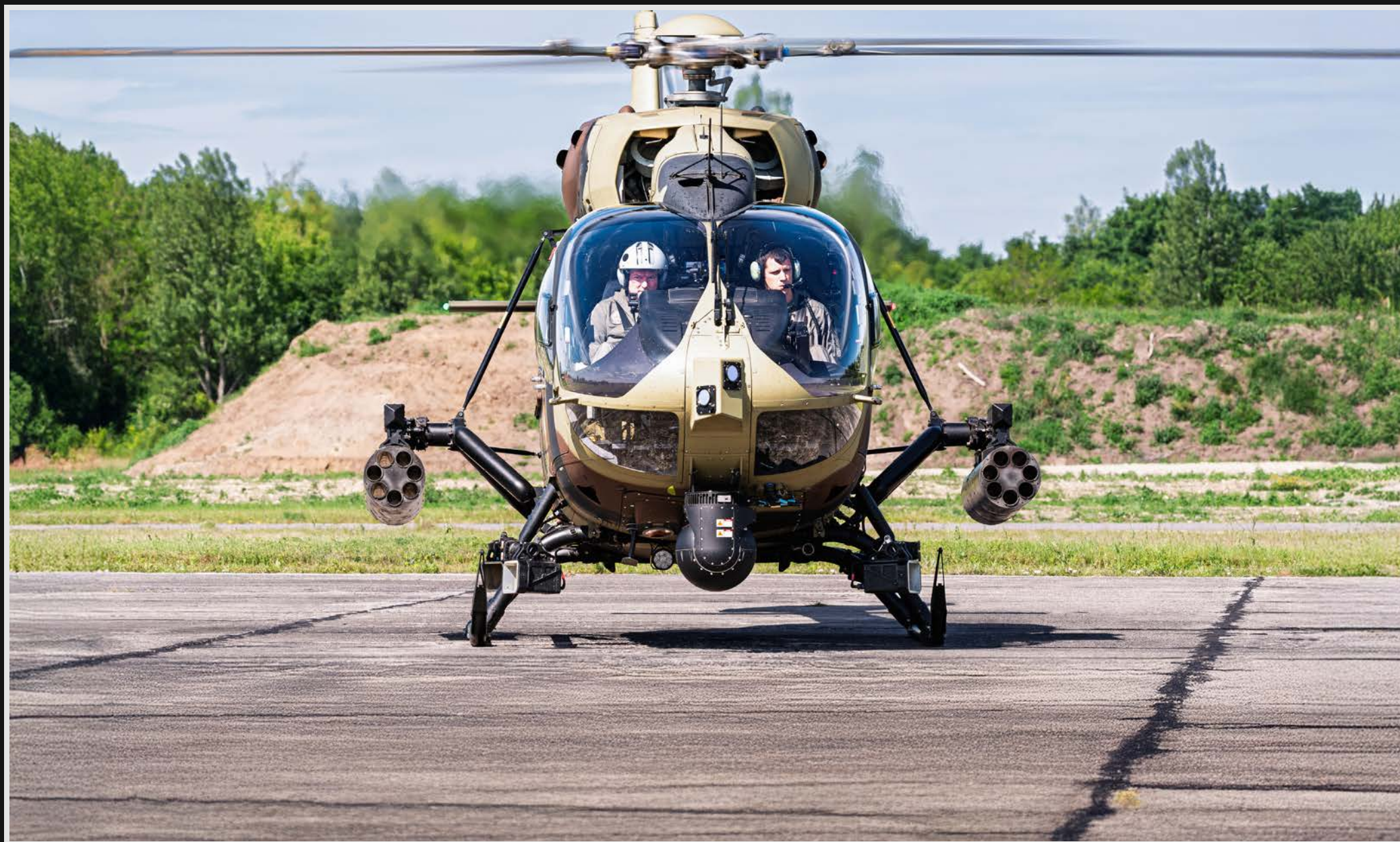
Integrated in the H145M's HForce modular weapon system is the Serbian-developed L-80-07 rocket launcher. This seven-tube launcher supports 80mm S-8KOM unguided rockets and is fully compatible with NATO and Russian-standard hardpoints
