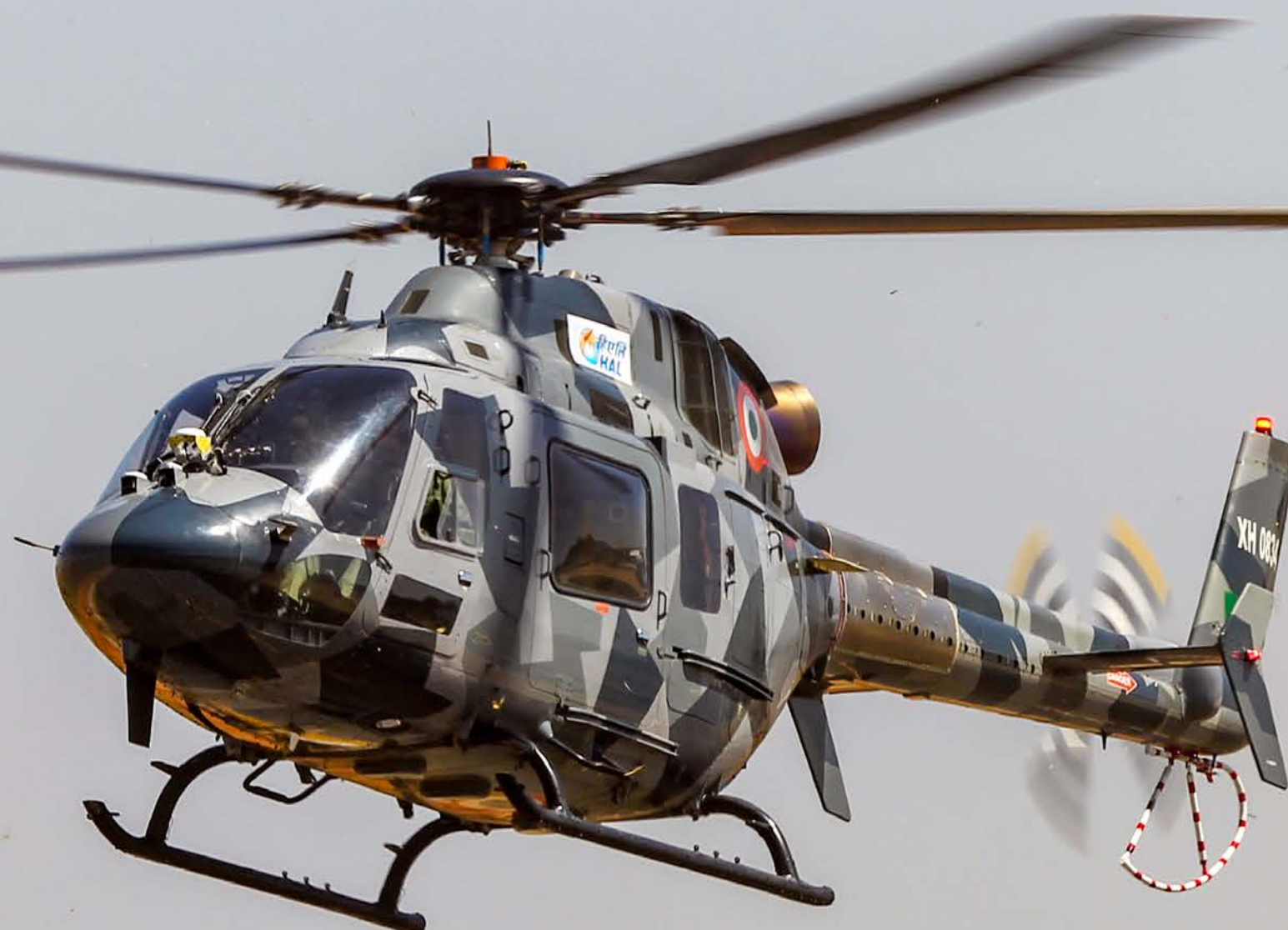
The Indian Air Force Light Utility Helicopter LHU – prototypes PT-3 (main), PT-1 (left), PT-2 (right) – is an indigenous helicopter developed by HAL for high-altitude and utility roles. Designed for troop transport, reconnaissance, and logistics, it features a glass cockpit, advanced avionics, and powerful Shakti-1U engines. The prototypes underwent extensive trials in varied terrains, including the Himalayas. LHU ensures reliable performance in extreme conditions and is a key element in replacing aging Cheetah and Chetak fleets.
