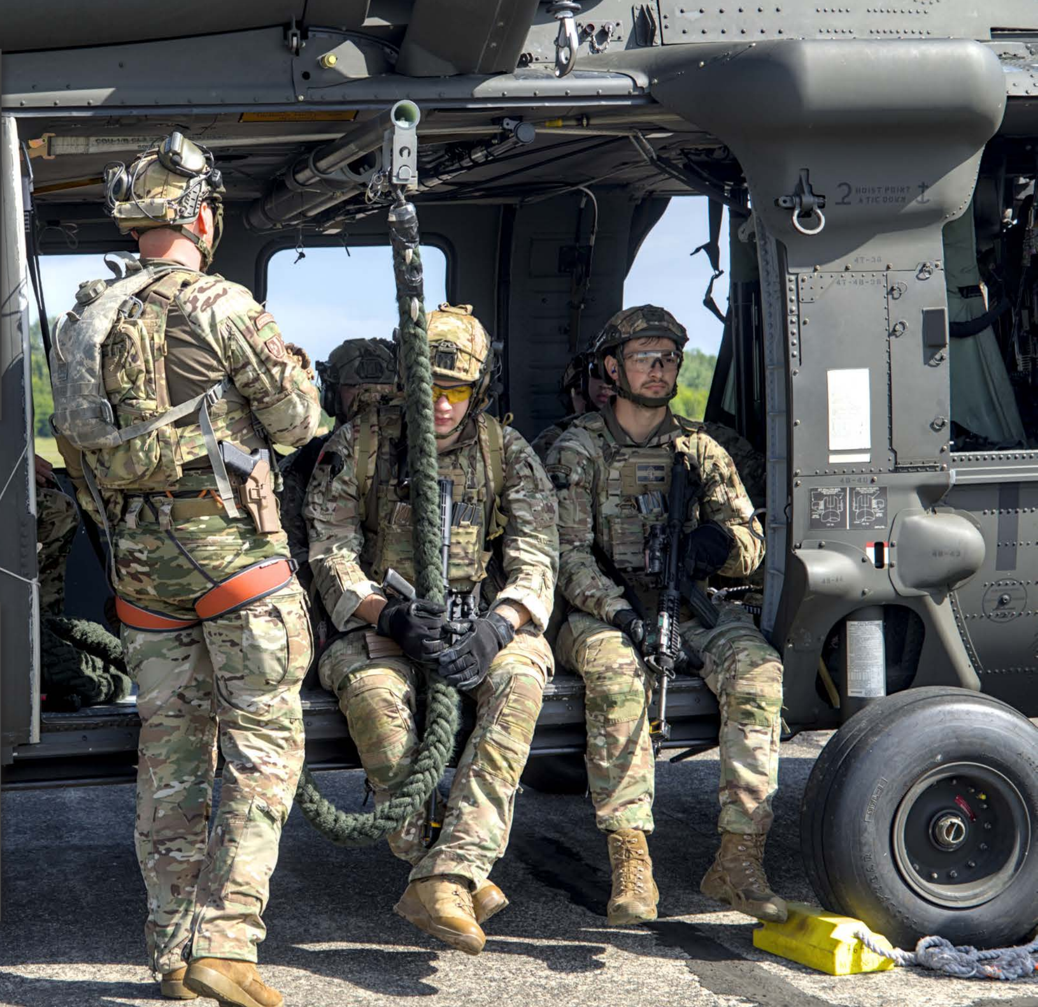
Members of the Special Forces wait inside the UH-60M for their go-order. The Black Hawk is equipped with a rope system that allows the soldiers to rappel (so called "fast roping") from the helicopter when landing is not possible – such as in rough or inaccessible terrain.
