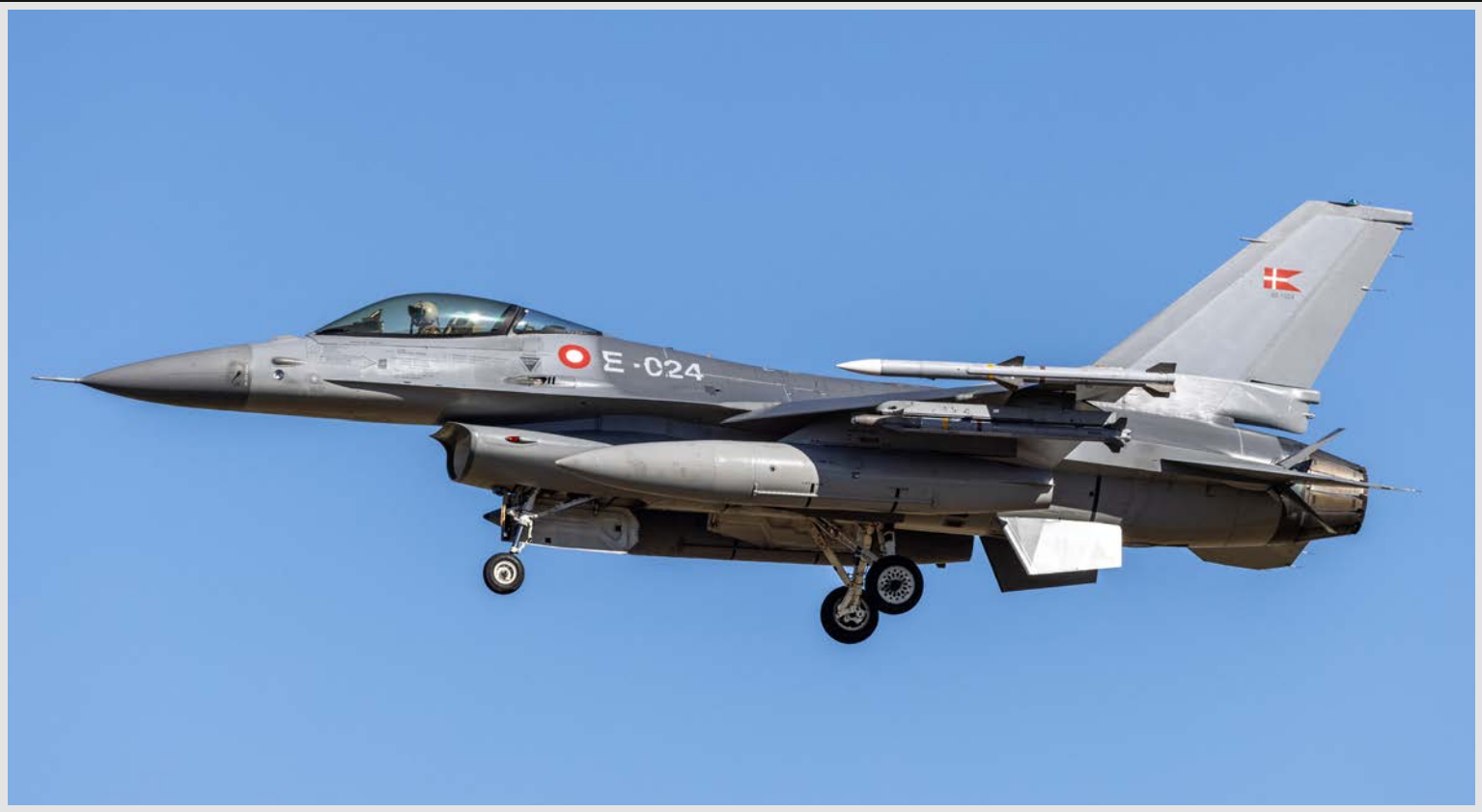
F-16AMs, E-024, ▲ and E-016 ▼ are outfitted with provisional markings applied as adhesive decals rather than permanent painted insignia. Such markings are commonly seen on aircraft in transitional phases, either en route to operational deployment or pending formal handover to a new air force, in this case the Ukrainian Air Force
