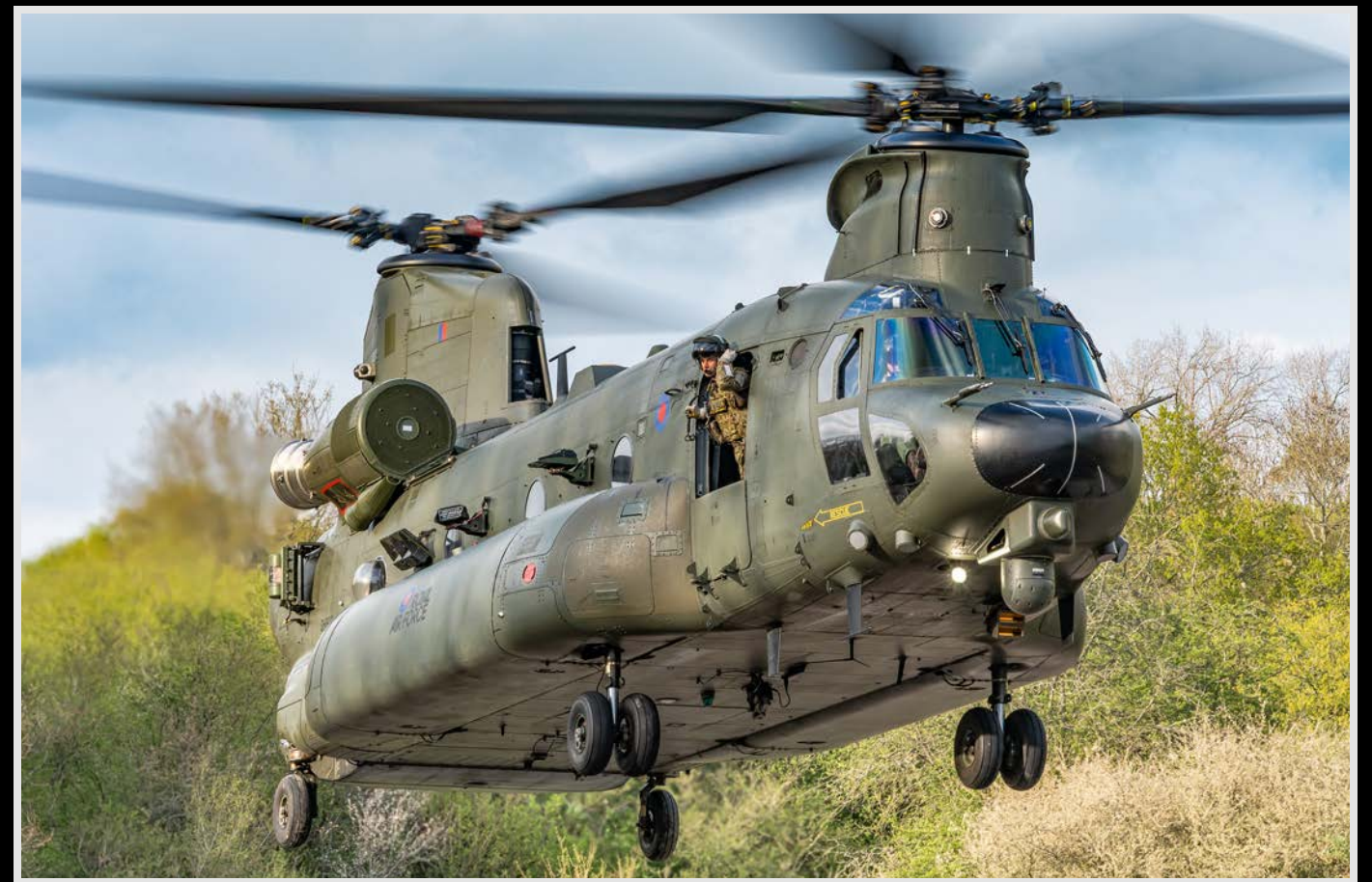
The HC5 variant of the Chinook is visually distinguished from the HC6 and HC6A models by its oversized, bulbous fuel tank
