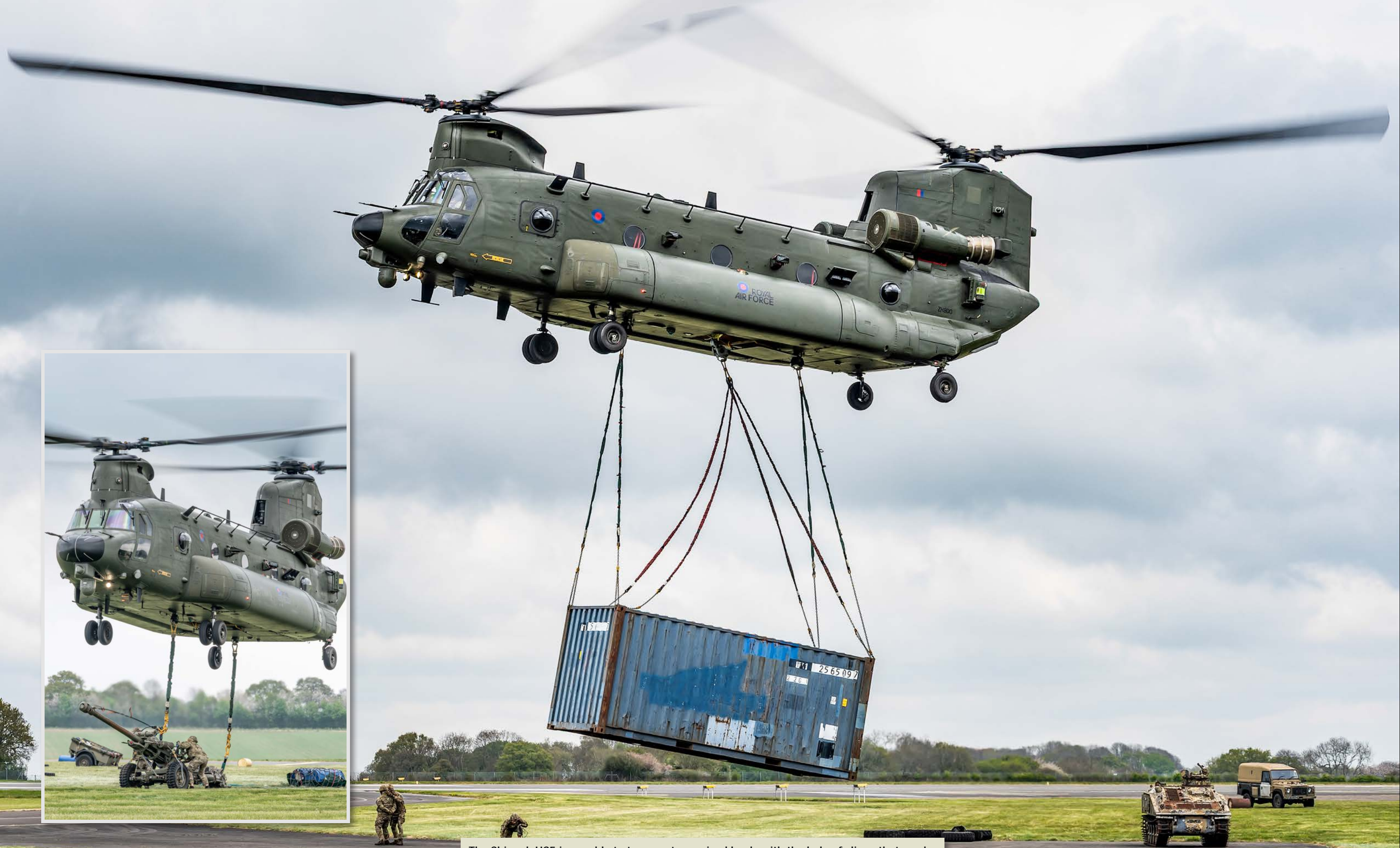
The Chinook HC5 is capable to transport oversized loads with the help of slings that can be attached to three external cargo hooks. The sling-load capacity is 26,000 lbs (11,793 kg) at the center hook, 17,000 lbs (7,711 kg) at the forward/aft hook, and 25,000 lbs (11,340 kg) tandem (for CH-47F)
