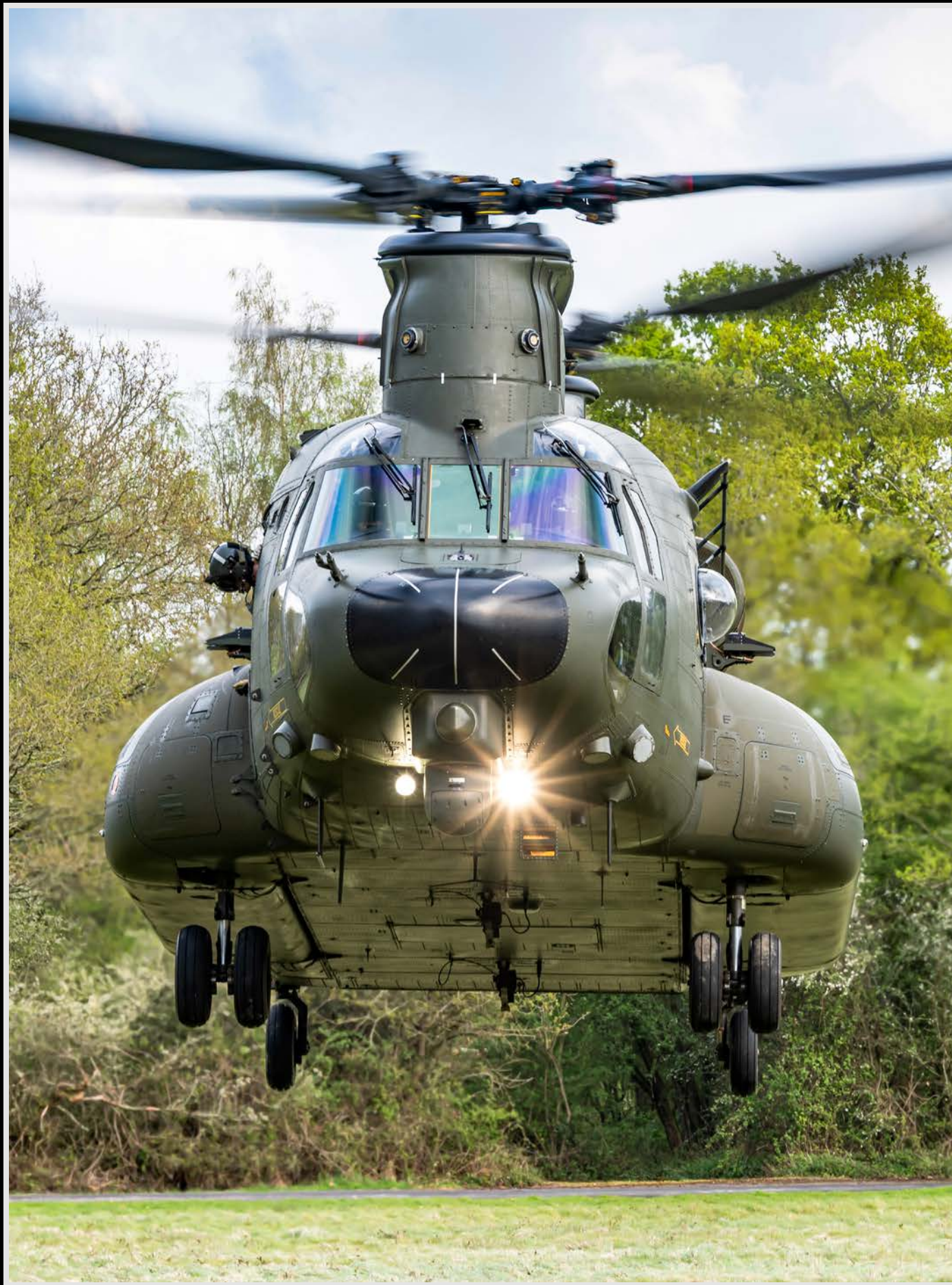
The HC5 variant of the Chinook is visually distinguished from the HC6 and HC6A models by its oversized, bulbous fuel tank
