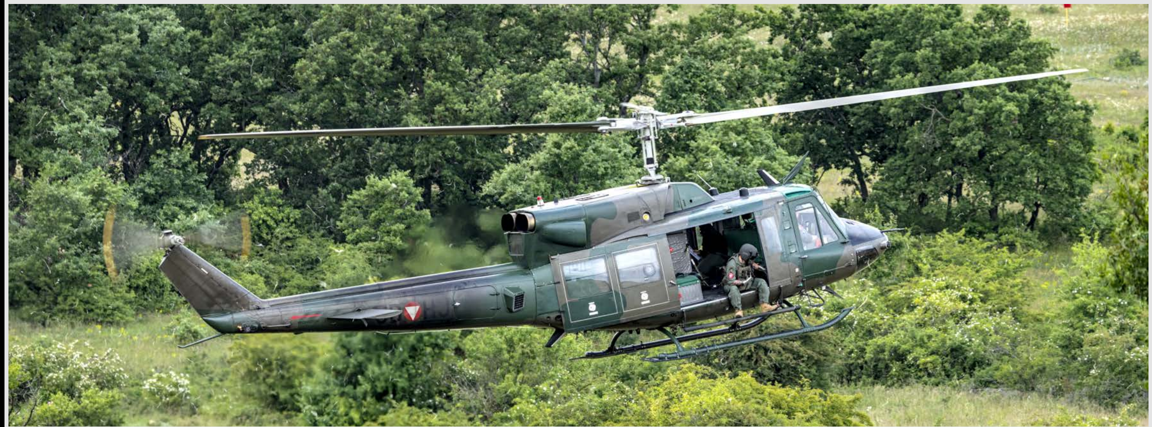
The Austrian Air Force AB212 can carry up to 14 passengers and has an external load capacity of 5,000 lb (2,268 kg). The helicopter has provisions for mounting MG 42/59 caliber 7.62 mm NATO machine guns on both sides of the fuselage
