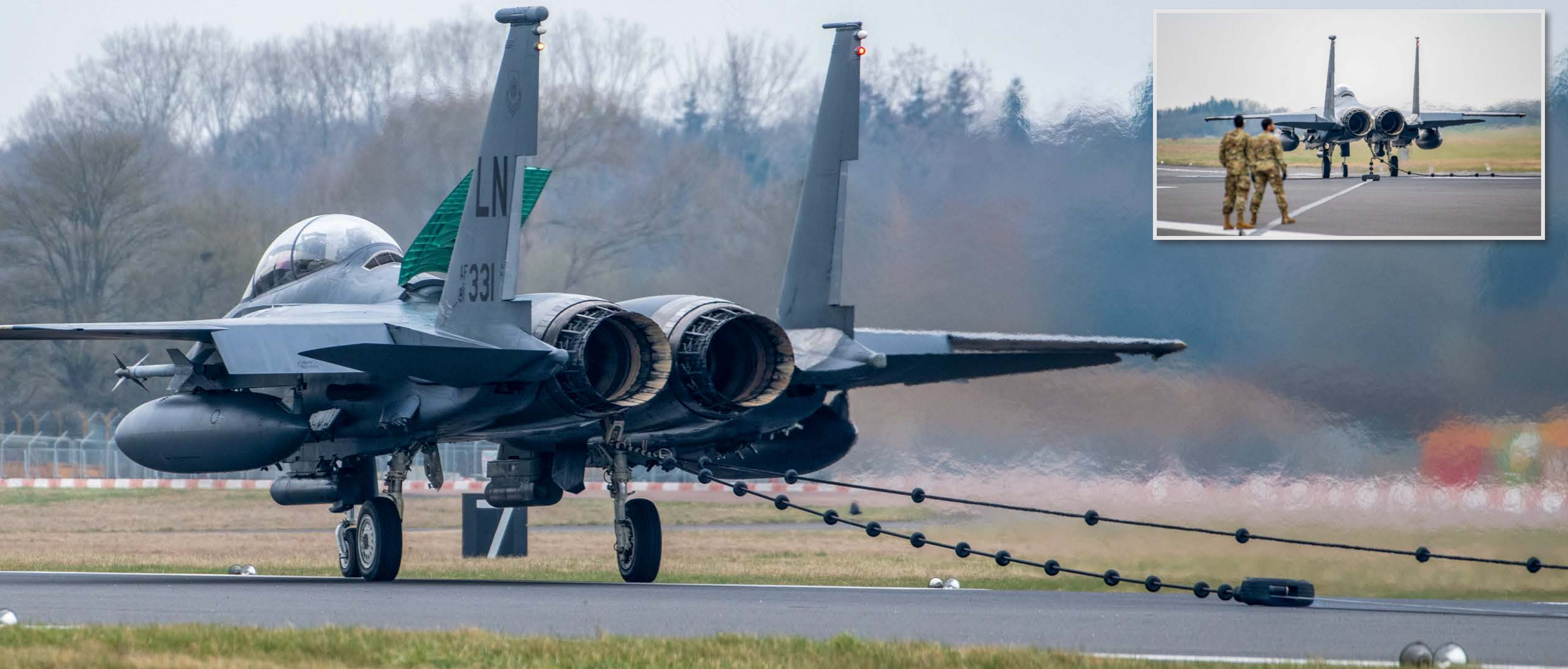
The F-15E Strike Eagle assigned to the 492nd Fighter Squadron tests a Mobile Aircraft Arresting System (MAAS) on RAF Fairford, England
