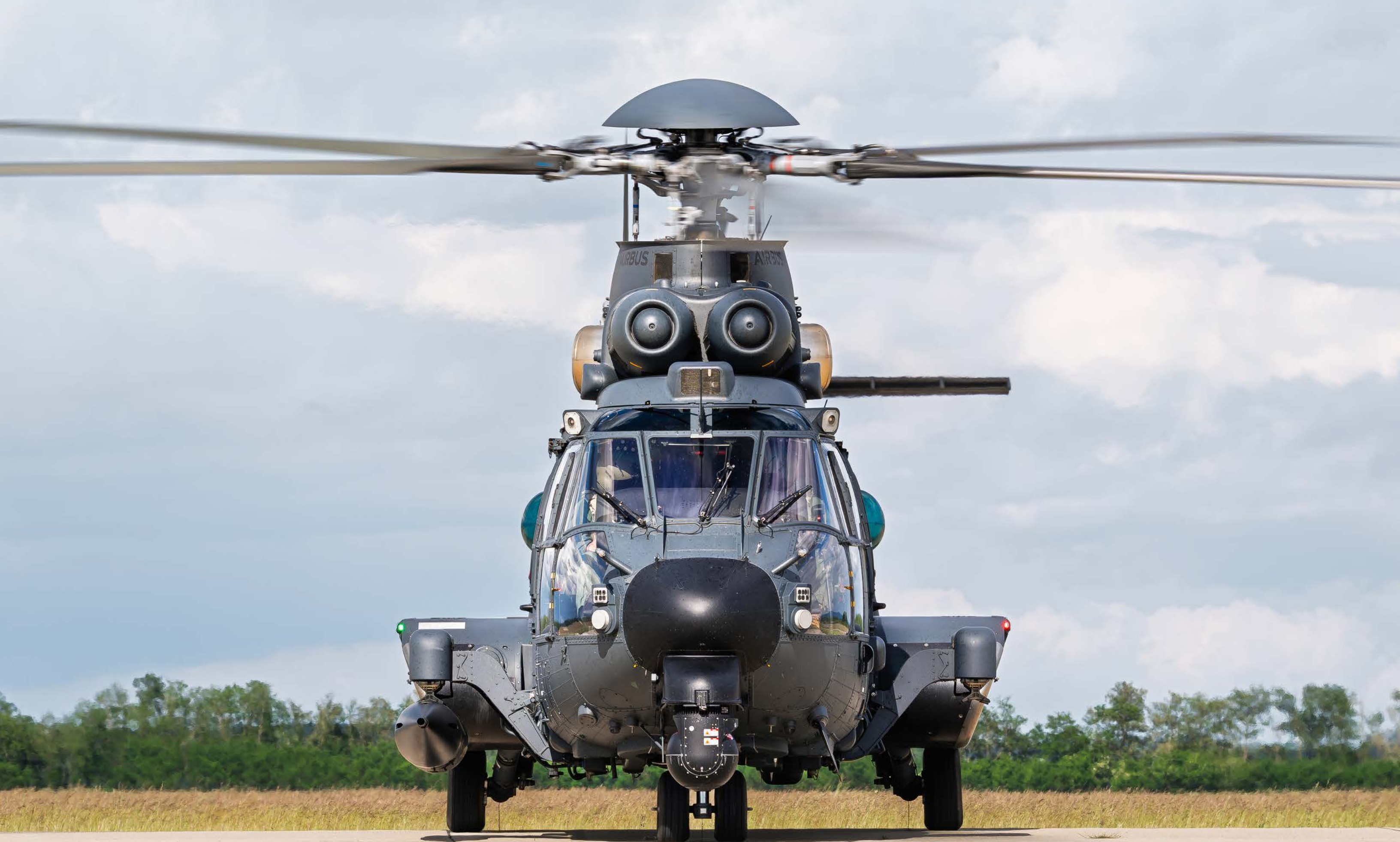
Head-on shot of a Hungarian Air Force H225M Caracal with a Nexter M621 gun pod attached to the starboard side of the helicopter
