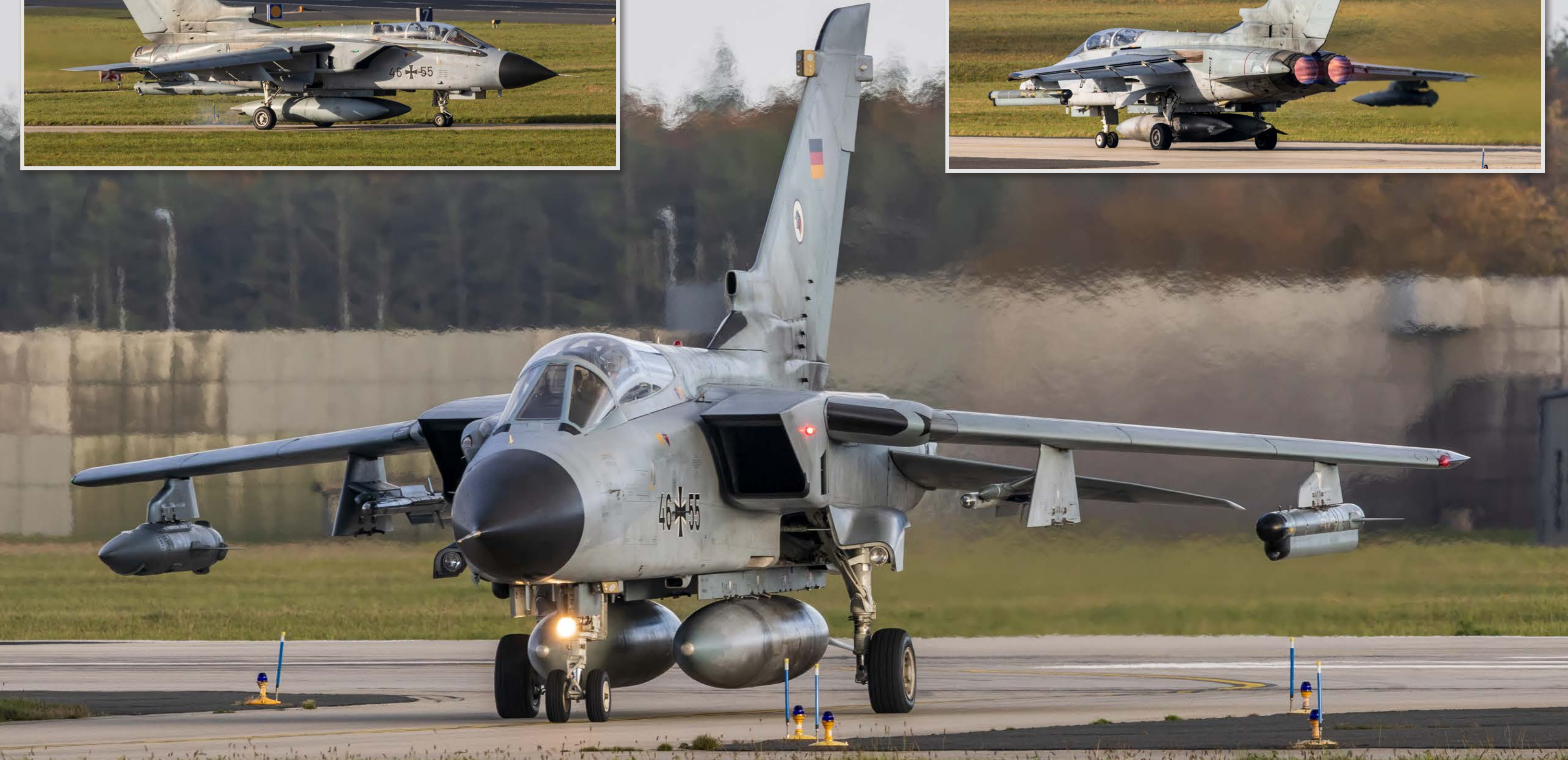
The Tornado ECR 46+55 flew in a very special configuration during the exercise. The 1,500 liter external tanks that are normally attached to the wings were attached to the fuselage. The two IRIS-T air-to-air guided missiles with infrared seeker heads for short and very short range can be seen on the wing's inboard stations
