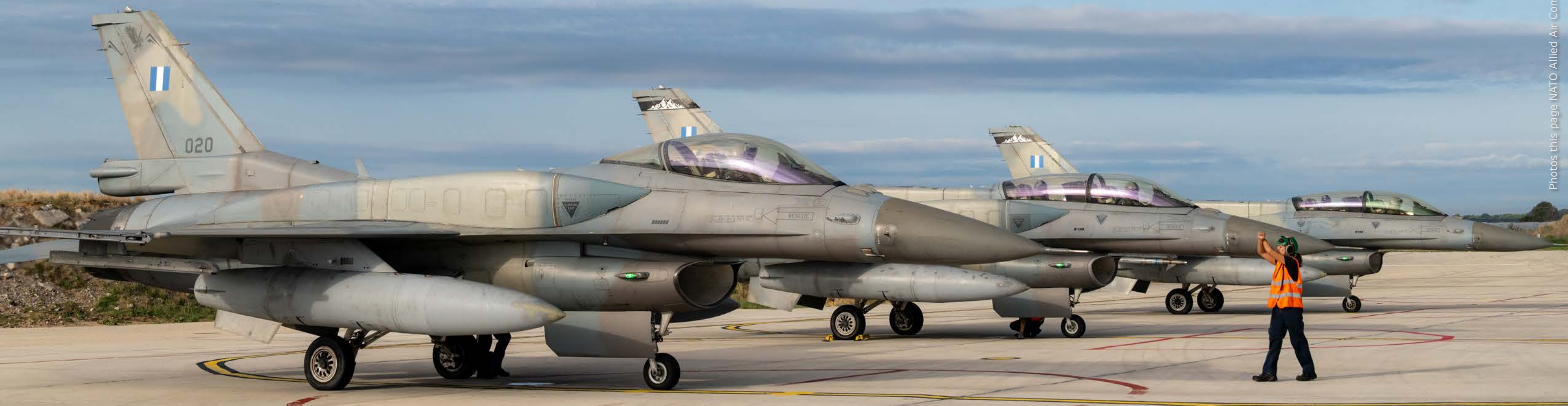
Hellenic Air Force F-16 Fighting Falcons assigned to 336 Mira at Araxos AB. The aircraft are fitted with CFTs (conformal fuel tanks). 'These external, pod-like fuel reservoirs are attached on the upper surface of the F-16's fuselage, with the tank's lower surface conforming to the aircraft shape. The upper surface arrangement allows the CFTs to be relatively light weight because nothing is suspended from them. With an empty weight of 900 pounds, tank set holds 450 gallons (ca. 3,050 pounds, or 2,271 litres) of additional JP-5/8 fuel. The extra fuel increases range, loiter time, and combat persistence as well as reduces the demand for tanker support. Range increase is on the order of twenty to forty percent, depending on the stores configuration and mission profile. The tanks have negligible effect on the aircraft agility, at subsonic speed. However, at supersonic speed, the drag is increased proportionally to the increase in speed. When fitted with CFT the aircraft retains almost the full handling qualities, flight limits, and signature. A complete set can be removed or replaced within two hours [...] set of CFTs carries 50 percent more fuel than the centerline external fuel tank, but has only 12 percent of the drag. The CFTs are designed for the full F-16 flight envelope – up to 9 g's, maximum angle of attack and sideslip and maximum roll rate' Source: Defense Update, Feb 4, 2024
