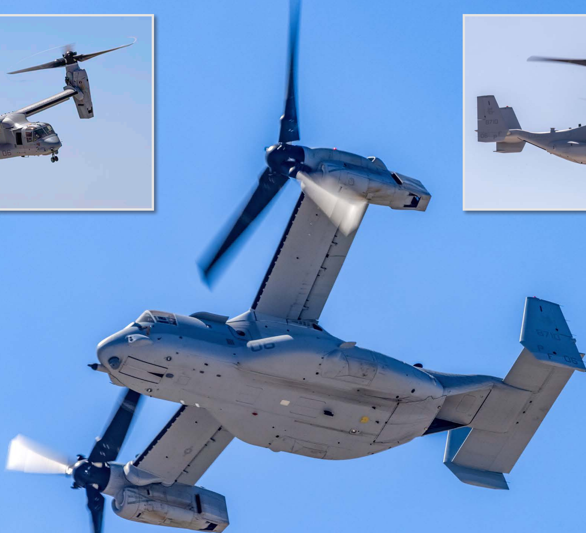
A U.S. Marine Corps MV-22B Osprey with Marine Medium Tiltrotor Squadron (VMM) 364, Marine Aircraft Group 39, 3rd Marine Aircraft Wing, performs a flight demonstration. With the speed and range of a turboprop, the maneuverability of a helicopter and the ability to carry 24 Marine combat troops twice as fast and five times farther than previous helicopters, the Osprey greatly enhances the advantages Marines have over their enemies. Main image and inset right USMC by Lance Cpl. Jennifer Sanchez
