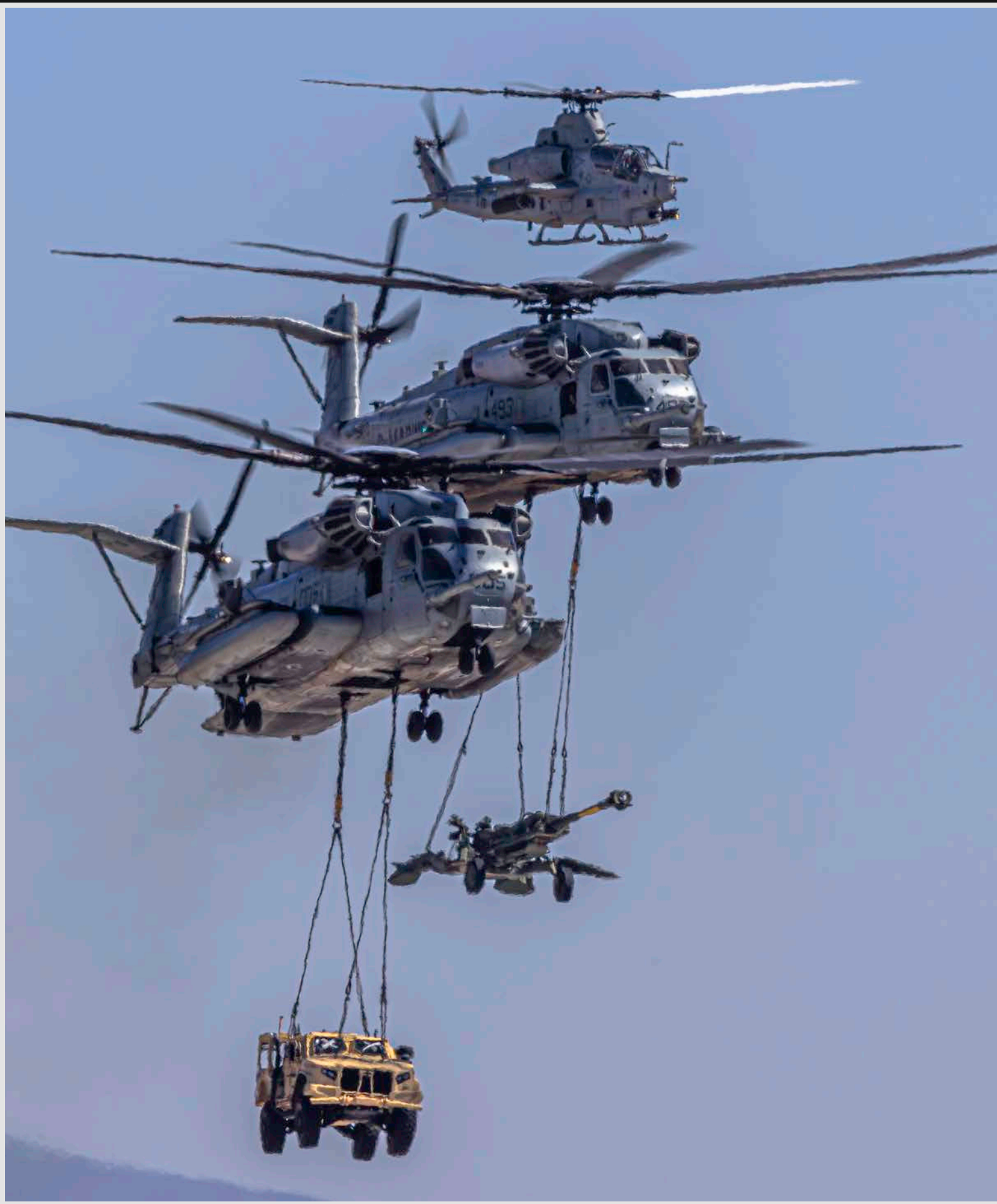
Left: AH-1Z Viper and two CH-53E Super Stallions carrying a 105mm M102 howitzer and a light armored M-ATV as an external sling load
