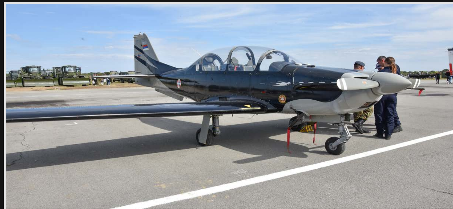
Lasta 95 (V-54) full-aerobatic military trainer aircraft with two wing hardpoints, assigned to 252. Shkolsko-Trenazhna Avijacijska Eskadrila (Training Aviation Squadron) (left) and to Tekhnicki Opitni Centar (Technical Test Center) (top and right)
