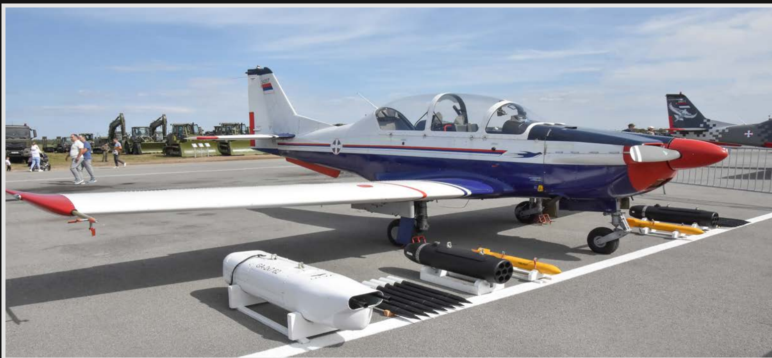
Lasta 95 (V-54) full-aerobatic military trainer aircraft with two wing hardpoints, assigned to 252. Shkolsko-Trenazhna Avijacijska Eskadrila (Training Aviation Squadron) (left) and to Tekhnicki Opitni Centar (Technical Test Center) (top and right)
