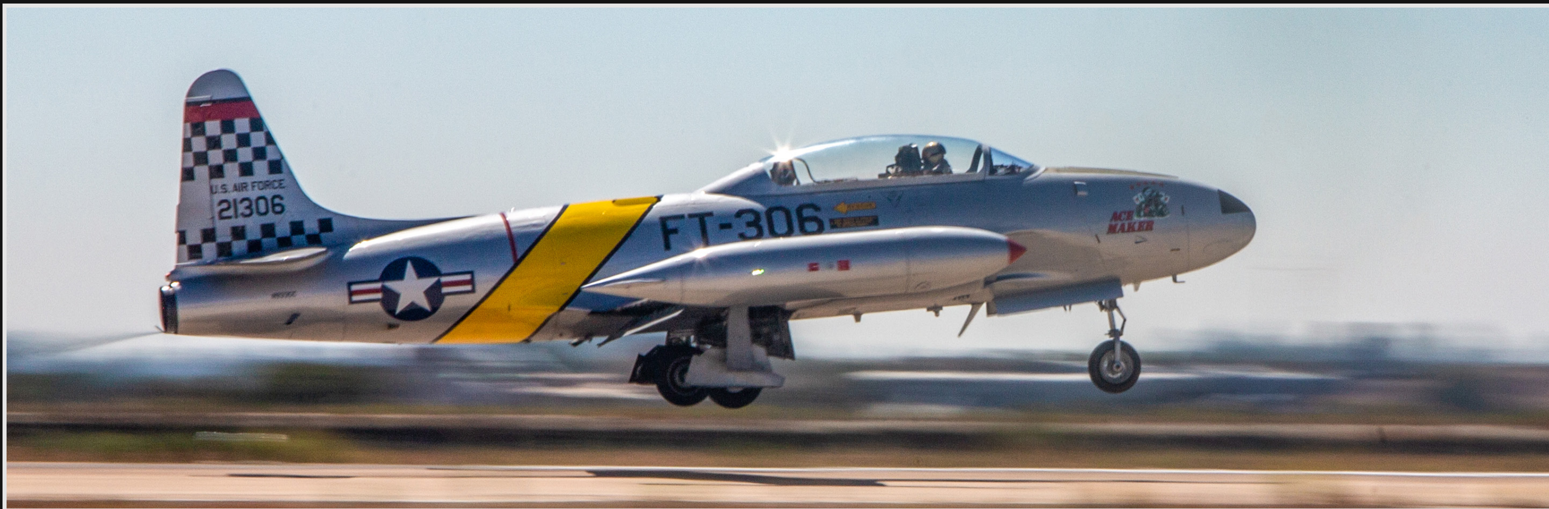
Lockheed T-33 Shooting Star . The T-33 was used as an subsonic jet trainer and made its first flight in March 1948. A total of 6,557 of this aircraft were manufactured between 1948 and 1959
