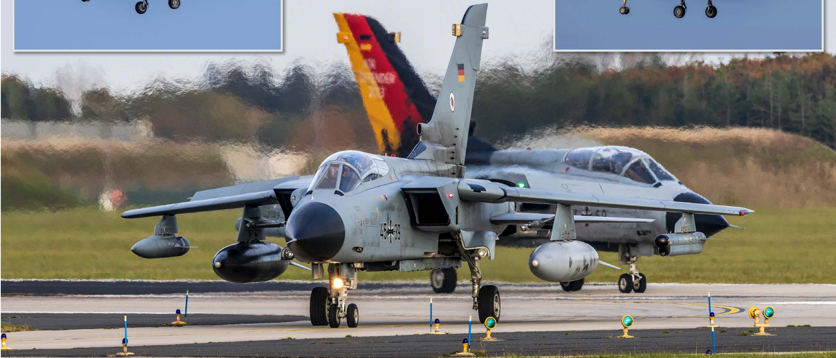
The Tornado 45+39 on final approach to Schleswig-Jagel AB and rolling off runway head no. 05. In addition to the two external tanks, the Tornado carries a BOZ-101 pod on the right outer station and a TSPJ pod (Tornado Self Protection Jammer) on the outer right station
