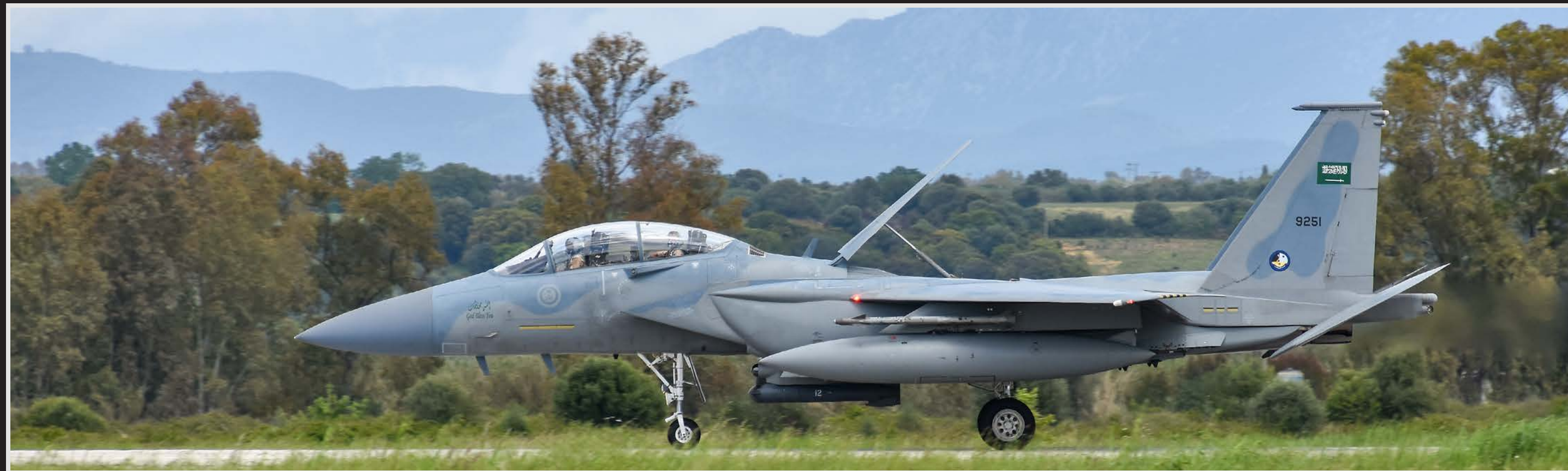
Saudi Arabian Air Force F-15SA Eagle assigned to 92 Squadron engages its speed brake to decelerate the aircraft after landing on the runway.
