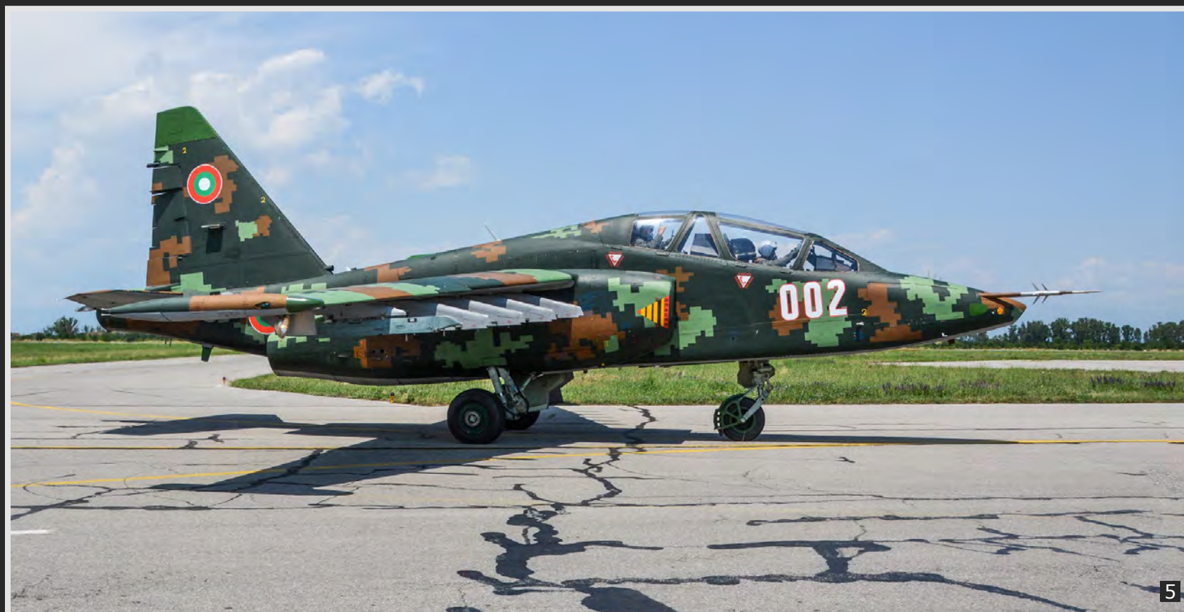
The Su-25K single-seat, twin-engine aircraft (serial 249) is designed for CAS (close air support). The trainer variant (serial 002) is designated Su-25UBK.
