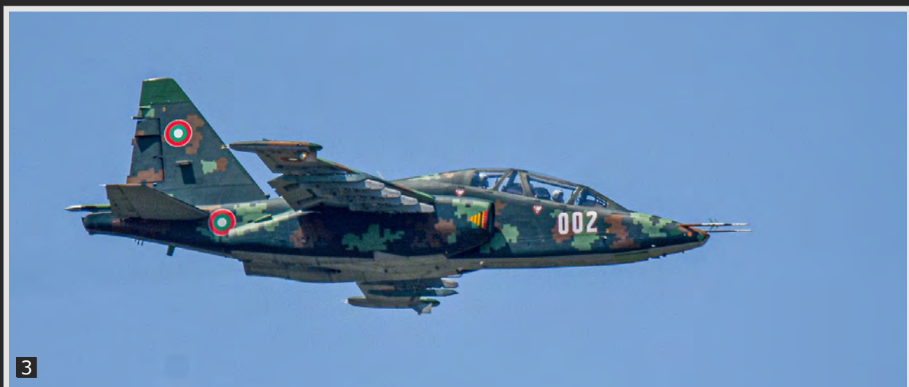
The Su-25K single-seat, twin-engine aircraft (serial 249) is designed for CAS (close air support). The trainer variant (serial 002) is designated Su-25UBK.
