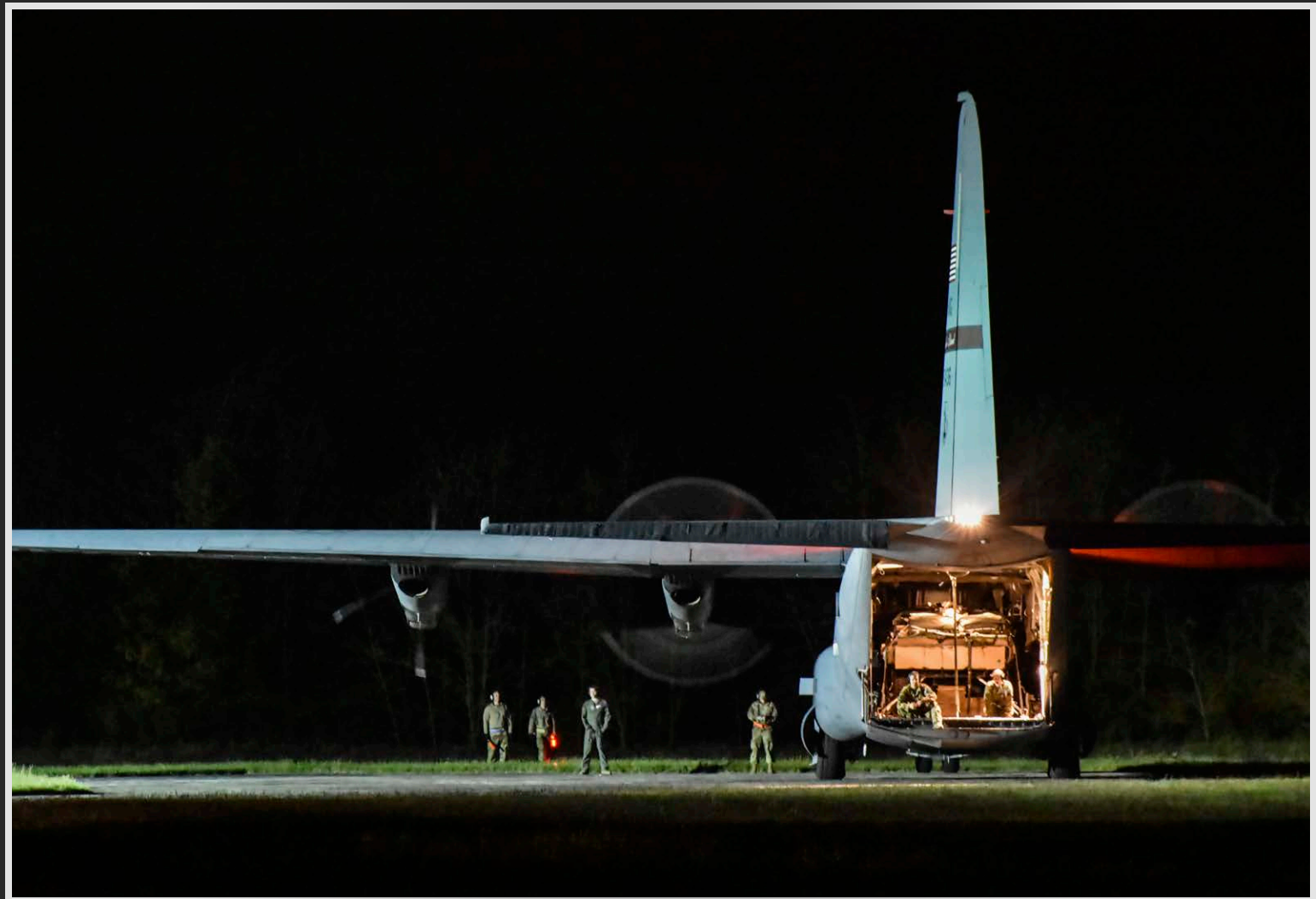
U.S. Air National Guard Lockheed C-130H Hercules assigned to 109th AS. Other than the C-17A, ▲ the C-130 is capable to deliver its cargo by dropping it in flight with the help of a parachute system. ▼
