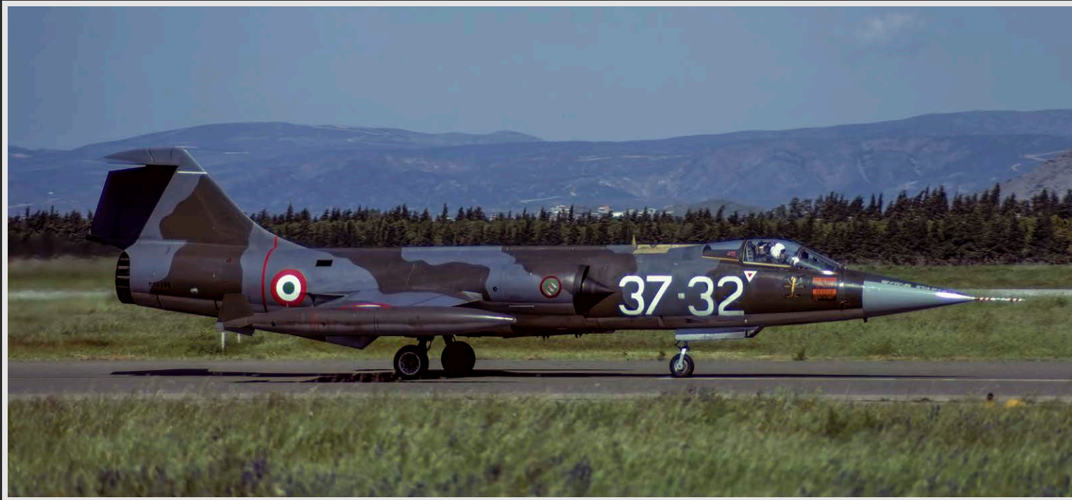
Italian Air Force Lockheed F-104S-ASA Starfighter assigned to 18° Gruppo/37° Stormo. Note the SUU-21 bomb dispenser for BDU48 and Mk75 bombs in addition to the fuel tip-tanks ( right ).
