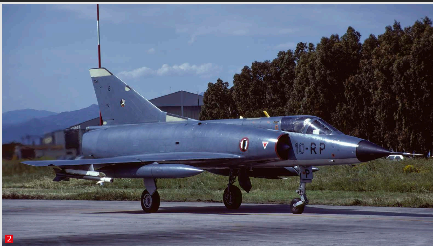
French Air Force Mirage IIIC assigned to EC 2/10 "Seine" at Creil AB, France with two external high speed fuel tanks and a Sidewinder sensor (1, 2, 3,) and with two large, standard fuel tanks (4).
