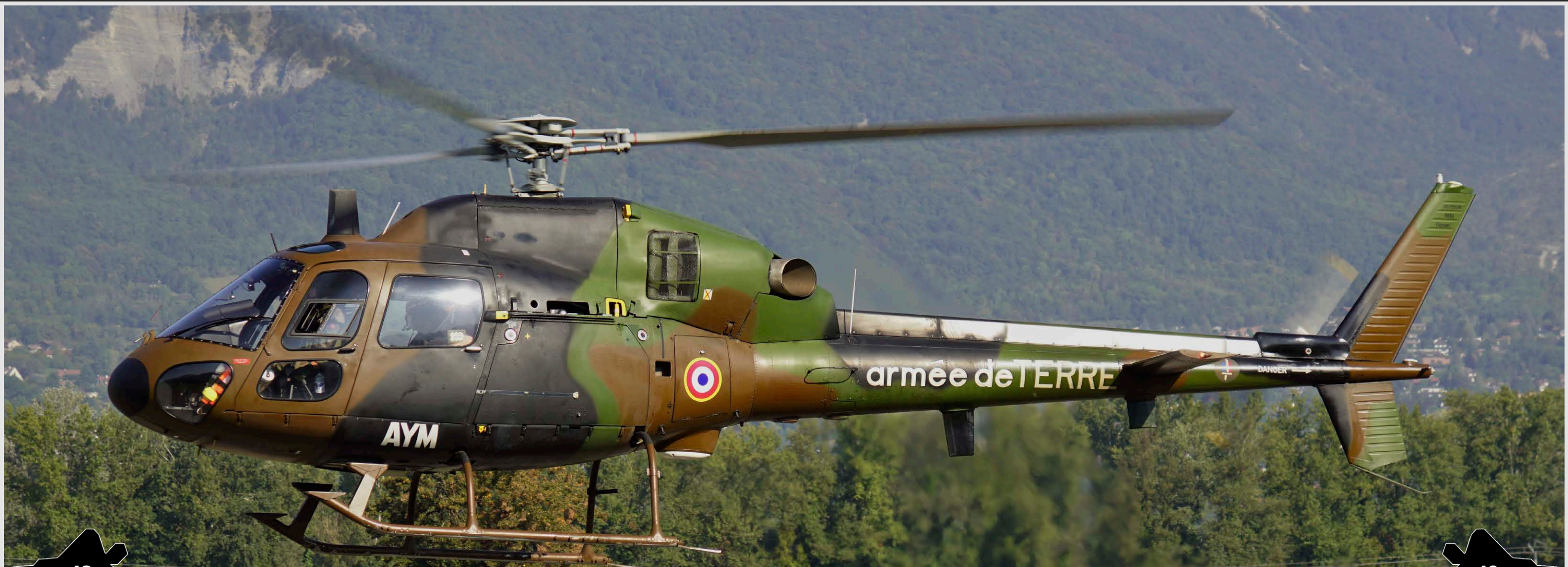
▲ AS342M Gazelle of the 5th RHC. It can be armed with four wire-guided anti-tank HOT missiles utilizing the SFIM APX M397 gyro-stabilized CCD/IR sight system.
