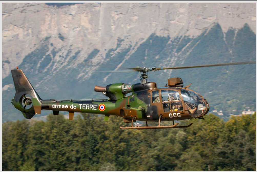
▲ AS342M Gazelle of the 5th RHC. It can be armed with four wire-guided anti-tank HOT missiles utilizing the SFIM APX M397 gyro-stabilized CCD/IR sight system.
