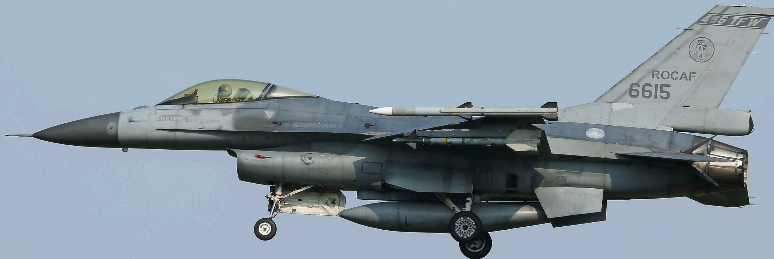
F-16A-20-CF assigned to the 21st TFG / 4th TFW at Chiayi AB. The aircraft is armed with live AIM-120 AMRAAM (at the wingtips) an AIM-9 Sidewinder (under the wing) air-to-air missiles.
