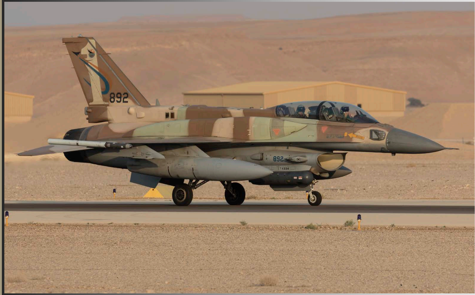
The F-16I Sufa is based on the F-16D and is heavily modified with Israeli-designed systems. Clearly visible are the Conformal Fuel Tanks (CFT) and the larger 600-gallons underwing fuel tanks. U.S. Air Force Europe F-16CM Wild Weasel assigned to 480th Fighter Squadron
