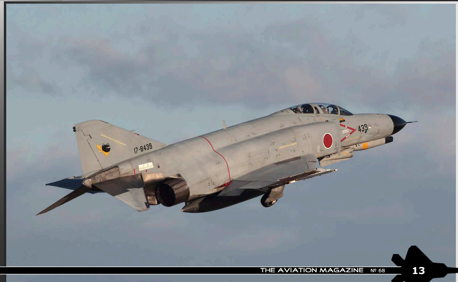
JASDF McDonnell Douglas F-4EJ Kai Phantom II . This is an upgraded version of the F-4EJ with improved avionics and ground attack capability.
