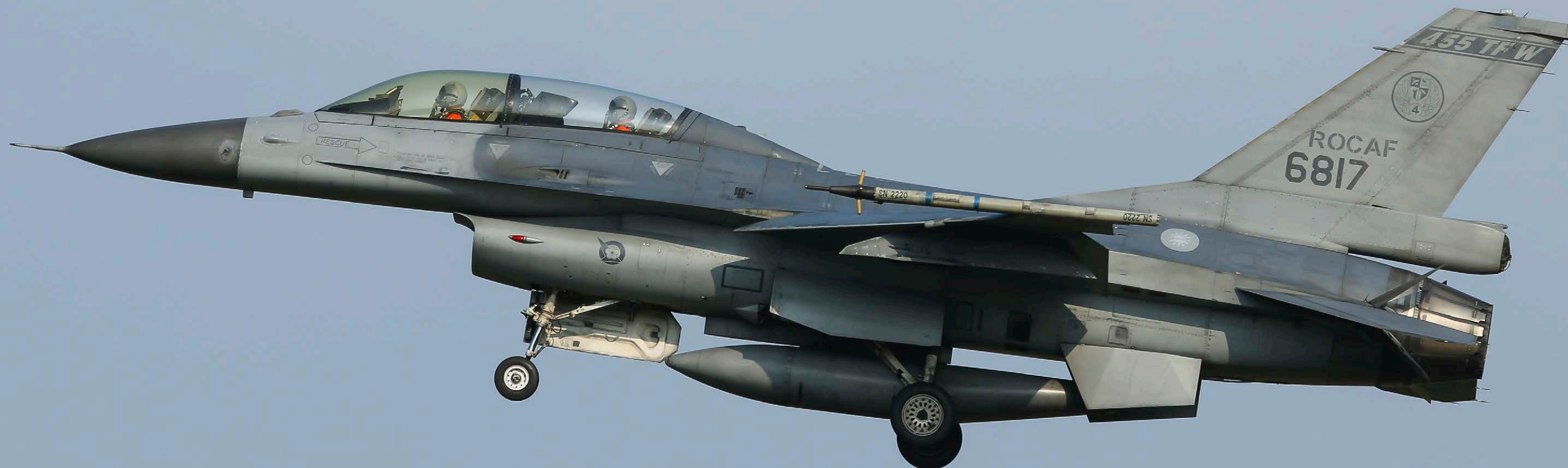
F-16B-20-CF assigned to the 23rd TFG / 4th TFW at Chiayi AB. The aircraft carries an Aircraft Instrumentation Subsystem (AIS) pod as part of the Tactical Aircrew Combat Training System / Air Combat Maneuvring Instrumentation (TACT/ACMI) system installed at the Taitung AB training range.
