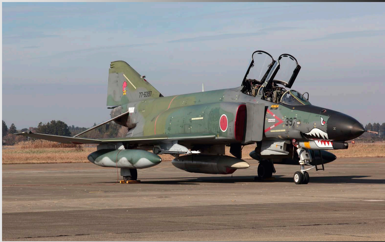
JASDF McDonnell Douglas F-4EJ Kai Phantom II . This is an upgraded version of the F-4EJ with improved avionics and ground attack capability.
