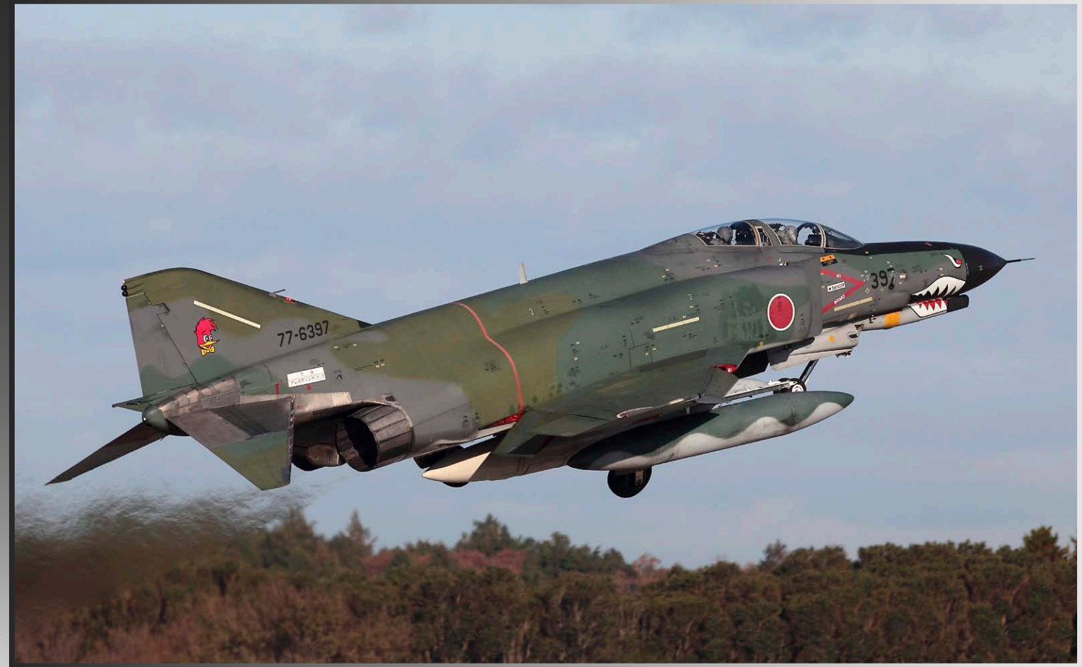
JASDF McDonnell Douglas F-4EJ Kai Phantom II . This is an upgraded version of the F-4EJ with improved avionics and ground attack capability.
